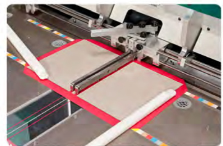
PräziCase Pro C1 Cutting the corners, turning-in all 4 edges, tucking-in the corner folds and pressing the complete book case
