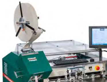
PräziSpine C1 Trimming flexible spine hollows from chipboard rolls
