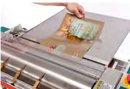
PräziCoat Pro C1 Gluing the cover material
